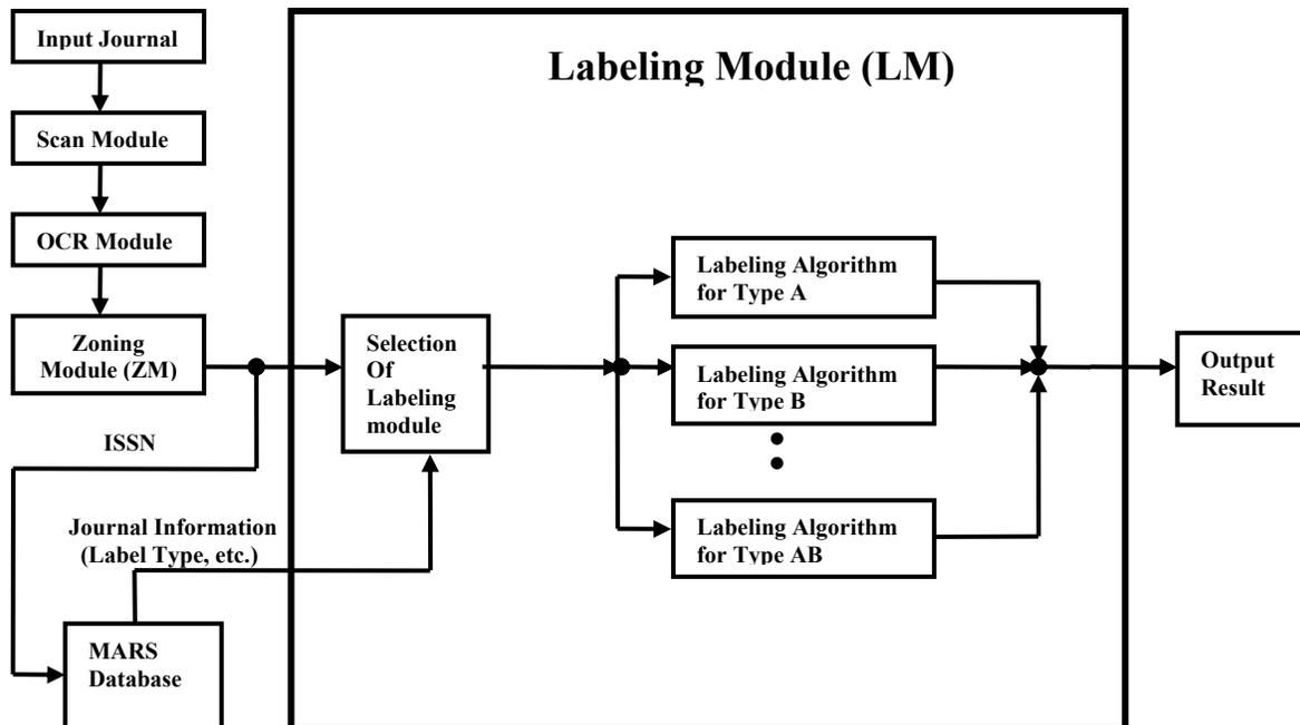
Figure 2. Structure of the Labeling module (LM).
