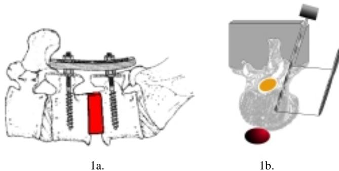
Figure 1. We are working on techniques for the precise placement of pedicle screws, required for many spine procedures. Figure 1a: lumbar plate secured with pedicle screws. Figure 1b: Our goal – a proposed template, guiding the drill path and depth. Structures such as the spinal cord, nerve roots, and the aorta must be avoided.
