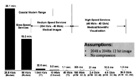
FIG. 4. Image transmission times.
