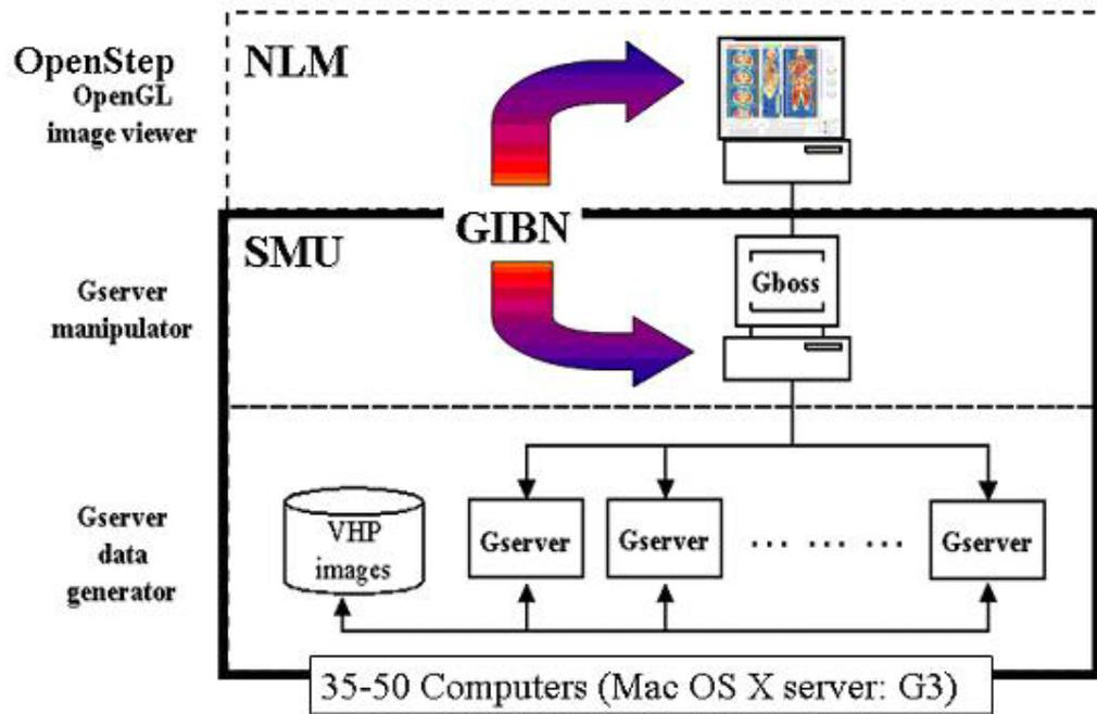
Fig. 3. The system of network multi-parallel computing
