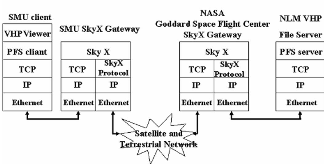
Fig. 6. Protocol stack of Remote Database Access Demonstration
