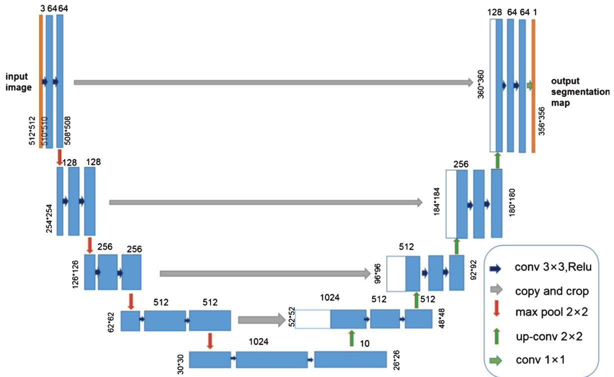
Fig. 3. Architecture of our adapted U-Net network.
