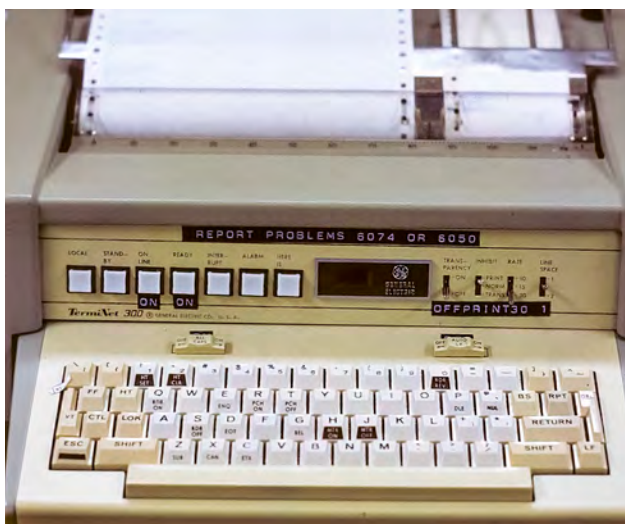
Printer, circa 1973, Regenstrief Institute. Used to print encounter forms, flowsheets summaries of patient EMR data, and reminder reports, the night before the patient's visit. The printouts were placed on the front of the patient's chart the day of their visit.
