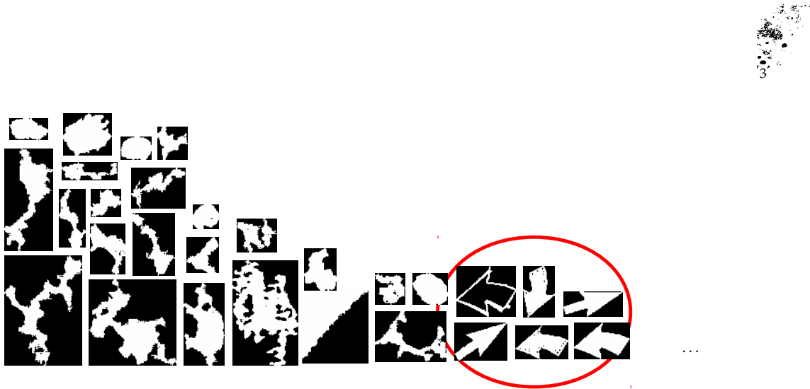
Figure 3. Fuzzy binarization (of Fig. 1 (c)): (a) four different levels (level 1 to level 4), where the segmented arrows are encircled both in red and black with respect to the background color; and (b) a collection of all segmented CCs including arrows (encircled in red).
