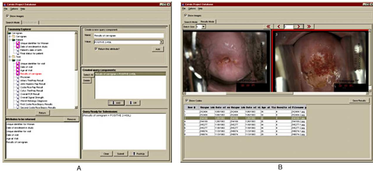
Fig. 18. Multimedia Database Tool. (A) Query-building screen with uterine cervix database tree; (B) results screen; records matching the query are returned. Text fields request by the user have their values returned in the table at the bottom of the screen. Corresponding images for each record are shown at the top of the screen in a horizontally-scrolled display.
