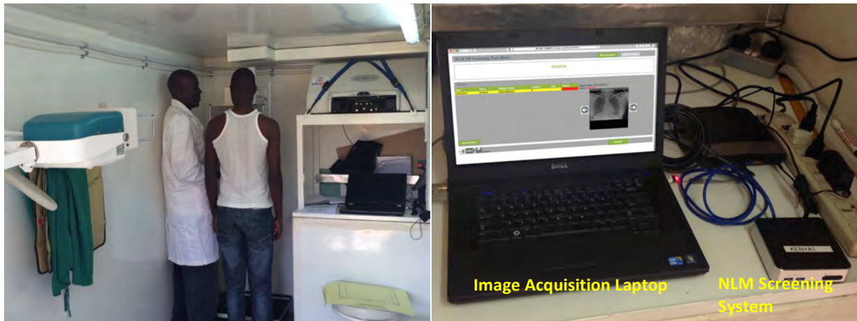
Figure 13. (Left) Radiographer Peter Otunga preparing a patient for X-ray imaging with X-ray cassette reader on shelf. (Right) On-board image acquisition laptop showing screening system UI, NLM Screening system (black box on the right), and router.
